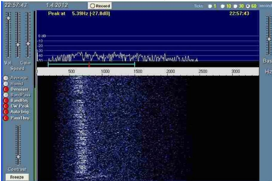
LX1DB\_01.04.2012\_20:57UT at OK1KIR (beam  $0.21^\circ$ ), spread  $\approx 150$  Hz, prediction  $\approx 418$  Hz (*libcalc VK3UM*)
