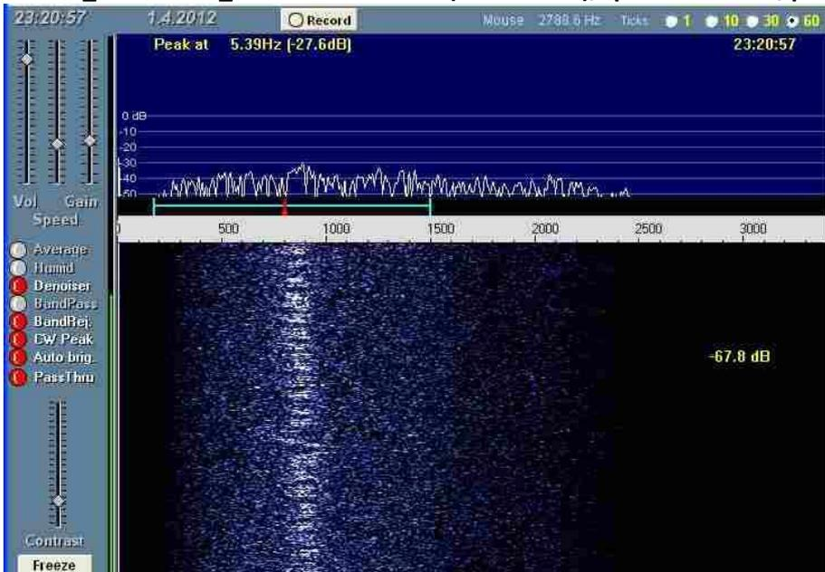
W5LUA\_01.04.2012\_21:20UT at OK1KIR (beam  $0.21^\circ$ ), spread  $\approx 100$  Hz, prediction  $\approx 257$ Hz (*libcalc VK3UM*)
