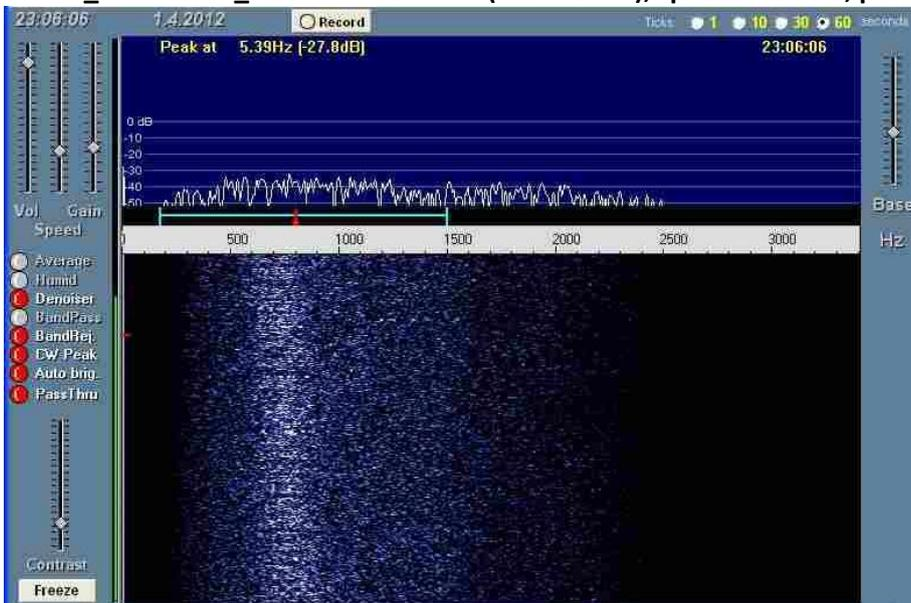
G4NNS\_01.04.2012\_21:06UT at OK1KIR (beam  $0.21^\circ$ ), spread  $\approx 200$  Hz, prediction  $\approx 411$  Hz (*libcalc VK3UM*)
